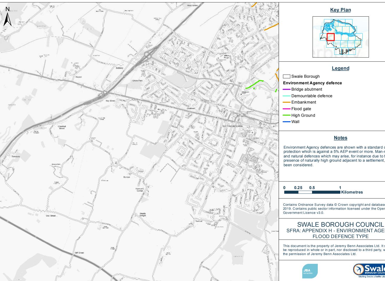
Environment Agency defences are shown with a standard of protection which is against a 5% AEP event or more. Man-made and natural defences which may arise, for instance due to the presence of naturally high ground adjacent to a settlement, have
